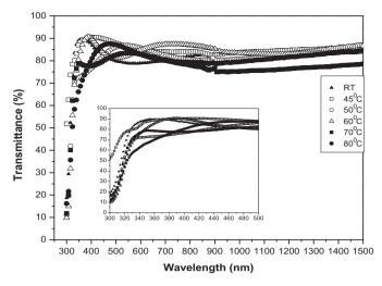
Fig. 11. Transmission spectra of CBD ZnS films deposited at different bath temperatures.
