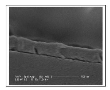
Fig. 4. SEM cross-sectional image of a typical ZnS film deposited under optimized conditions.
