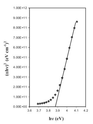
**Fig. 10.**  $(\alpha h\nu)^2$  Versus  $h\nu$  plot for a typical CBD ZnS film deposited under optimized conditions: [ZnSO<sub>4</sub>] = 0.05 M, [TA] = 0.04 M, [NH<sub>3</sub>] = 9.8 M and  $t_b = 60$  °C.
