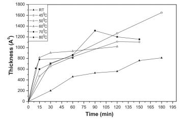
Fig. 1. Thickness variation as a function of time at different bath temperatures. Bath composition:  $[ZnSO_4] = 0.05 \text{ M}$ , [TA] = 0.02 M,  $[NH_3] = 9.8 \text{ M}$ .
