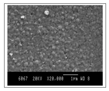
Fig. 6. SEM image of a typical ZnS film deposited under optimized conditions.
