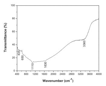
Fig. 8. FTIR spectrum of a typical ZnS film deposited under optimized conditions: [ZnSO<sub>4</sub>] = 0.05 M, [TA] = 0.04 M, [NH<sub>3</sub>] = 9.8 M and  $t_b$  = 60 °C.
