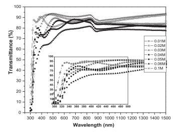
Fig. 9. Transmission spectra of CBD ZnS films deposited with different thioacetamide concentrations. Inset: Expanded view of the fundamental absorption region.
