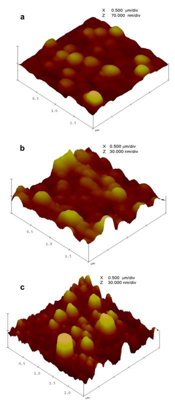
**Fig. 7.** AFM images of CBD ZnS films deposited from chemical baths with different thioacetamide concentrations keeping  $[ZnSO_4] = 0.05$  M,  $[NH_3] = 9.8$  M and  $t_b = 60$  °C. (a) [TA] = 0.02 M, (b) [TA] = 0.04 M, (c) [TA] = 0.06 M.
